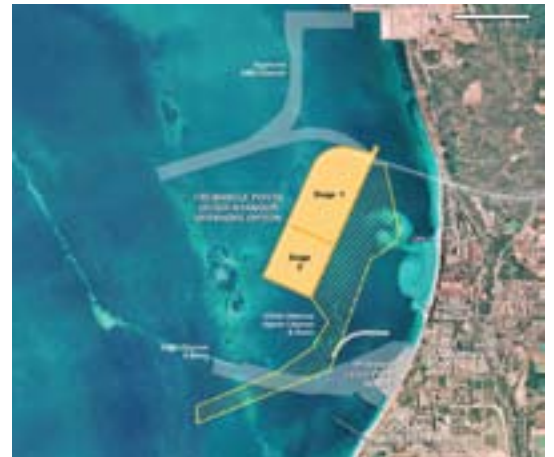
OUTER HARBOUR Option 1 (above): An offshore island linked to shore by 1 km rail and road bridge.
