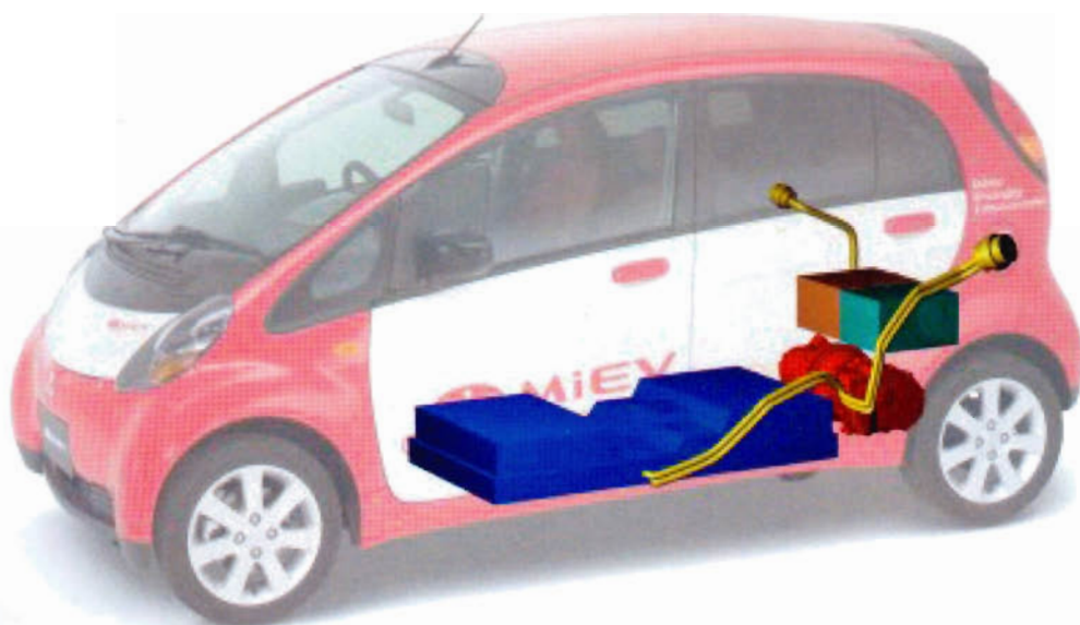
X-ray view of the iMiEV's 47kw electric motors (red) and its 330-volt lithium-ion batteries (blue).
